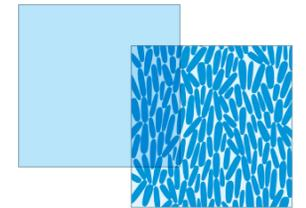
Lithium disilicate crystallites 2000-4000nm
