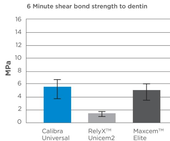
Test: Shear Bond Strength to dentin after self-curing for 6 minutes at 37°C. Source: Dentsply Sirona.
