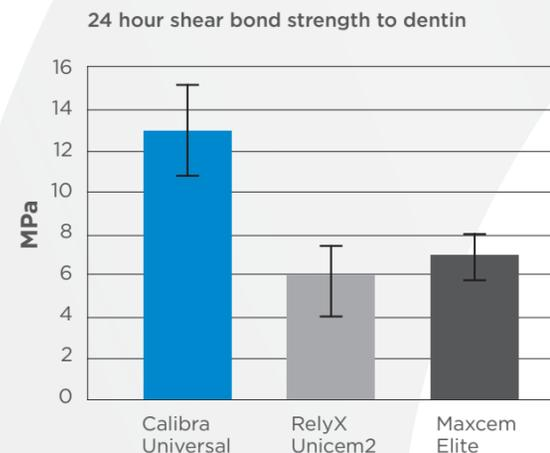
Test: Shear Bond Strength to dentin after self-curing for 24 hours at 37°C. Source: Dentsply Sirona.
