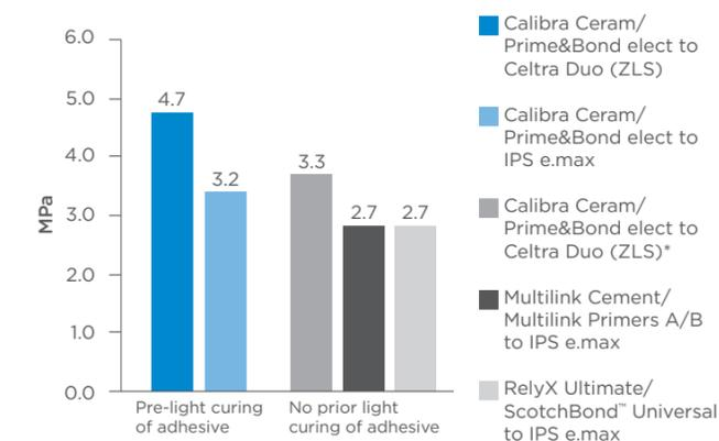
Test: Crown-pull Bond Strength Testing. Ceramics were treated with 5% HF and silanated. All adhesives were used in self-etch mode. All cements were self-cured except for the group with optional light-curing through crown. Artificial aging: 10,000 thermocycling (5-55°C). Source: Prof. John Burgess.
