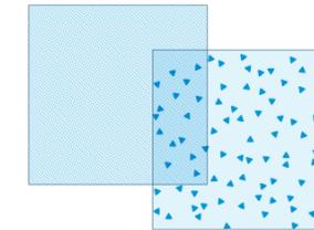
Lithium silicate crystallites 500-700nm
