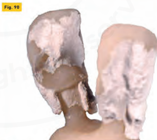
[Fig. 90] After water divesting there is a little investment for sandblasting left.
